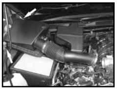
Step 4 Release the two clips securing the top of the air box and remove the air box intake tube assembly from the vehicle. Remove the stock air filter.
