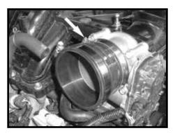
Step 11 Install the supplied coupler onto the throttle body and secure with the supplied hose clamp.
