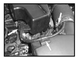
Step 2 Disconnect the mass air meter
