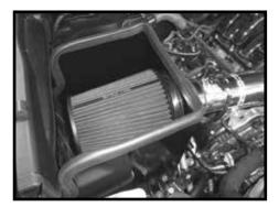
Step 13 Install the air filter onto the velocity stack adapter and secure with the supplied hose clamp. Then re-install the engine cover.
