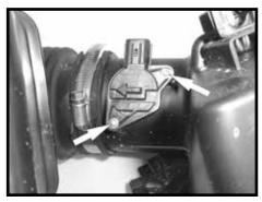
Step 7 Remove the two screws securing the mass air meter sensor to the stock intake tube and then remove the sensor.
