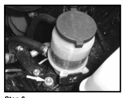
Step 6 Remove the bolt that secures the power steering reservoir to the vehicle. The screw will be reused in step 10.
